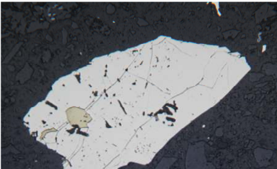
Sample 3-1. Pyrite with chalcopyrite inclusions. Field of view = 1.35 mm.
