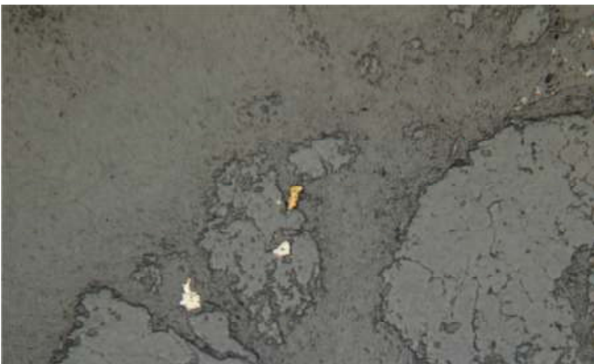
Sample 2.. Small gold(?) and pyrite grains. Field of view = 1.35 mm.
