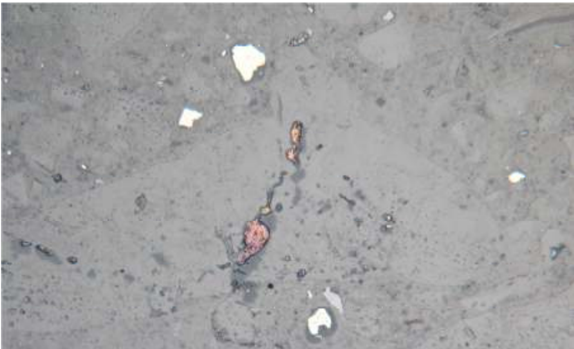
Sample 1-1. Seam of gold-electrum in quartz. Pyrite grains and sphalerite in bottom center. Field of view = 1.35 mm.
